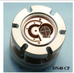
Top view of the 3BG-03, without the cover on the deflector and collector. The flanged mounting surface of the deflector can be seen in the picture, with its 3 mounting holes. Within the functional volume of the gauge, the deflector is an open array of bars and slots.
